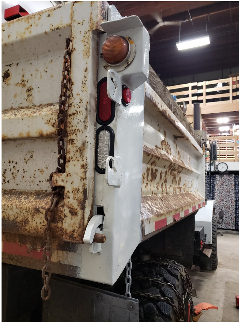
Fabricated Tail Light Holders on Osh Kosh Dump Truck
